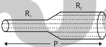
$$R = \frac{8\eta l_1}{\pi r_1^4} + \frac{8\eta l_2}{\pi r_2^4} \text{ and } Q = \frac{P}{R_1 + R_2}$$
