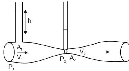
$$\text{Velocity of flow } V_1 = \sqrt{\frac{2gh}{\left(\frac{A_1}{A_2}\right)^2 - 1}}$$
