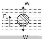
c) **Terminal velocity** : When a body is dropped in a fluid at one stage the resultant force acting on it will be zero and it travels with uniform velocity and this is called terminal velocity.
