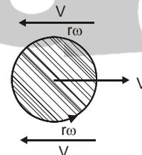
76. If the ball is moving from left to right and also spinning about a horizontal axis perpendicular to the direction of motion, then relative to the ball air will be moving from right to left. The resultant velocity of air above the ball will be v+rω while below it v-rω. So in accordance with Bernoulli's principle pressure above the ball will be less than below it. Due to this difference of pressure an upward force will act on the ball and hence the ball will deviate from its usual path.
