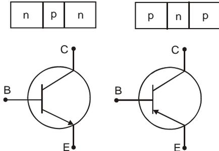
33. Transistors are of two types i) n-p-n, ii) p-n-p
