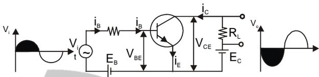
44. The process of raising the strength of weak signal is known as amplification and the device which accomplishes this job is called amplifier. The phenomenon of amplification is necessary in radio communication systems.
