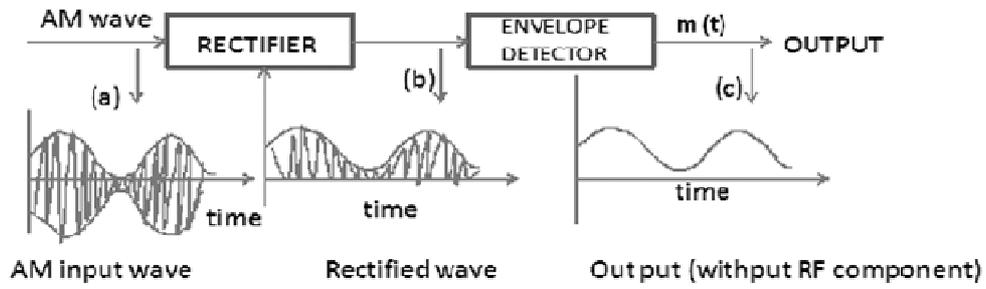
The modulated signal of the form given in (a) of fig is passed through a rectifier to produce the output shown in (b). This envelope of signal (b) is the message signal. In order to retrieve  $m(t)$ , the signal is passed through an envelope detector (which may consist of a simple RC circuit).
