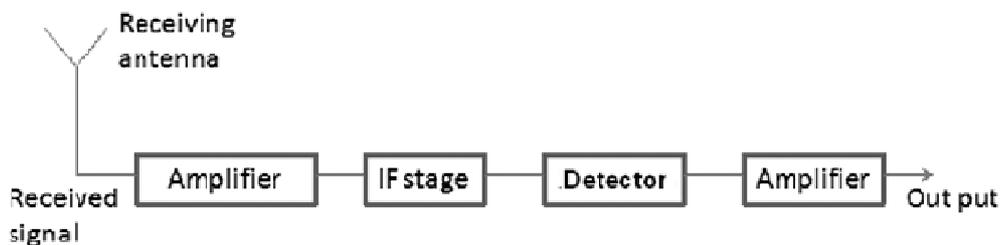
The IF signal contains the frequencies  $\omega_c$  and  $\omega_c \pm \omega_m$ . To obtain original message signal  $m(t)$  of angular frequency  $\omega_m$ , simple AM detector is shown in diagram.
