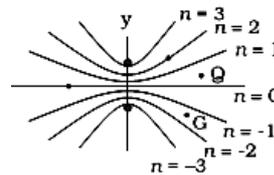
Locus of points for which  $S_1P - S_2P$  is equal to zero,  $\pm\lambda$ ,  $\pm 2\lambda$ ,  $\pm 3\lambda$ .
